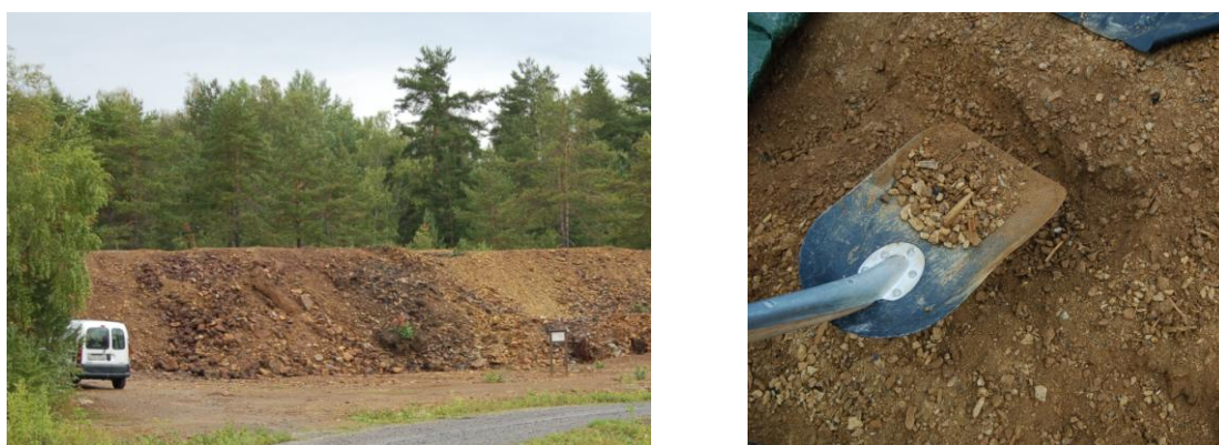
Figure 3-2. Rock waste deposit at Ljusnarsberg mine site (left) and close – up photo of weathered, acidic rock waste that requires treatment.
