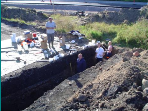
MSWI slag road is examined after 18 years of use.
